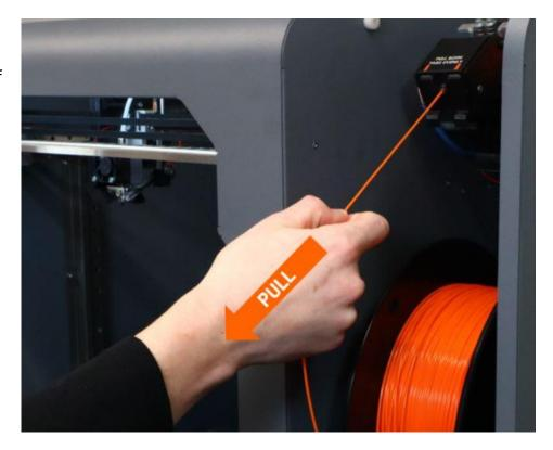
4. Spin the spool in reverse to wind up the length of filament that was ejected from the extruder. Then tuck the end of the filament into the side of the spool; most spools have small holes for this purpose.
