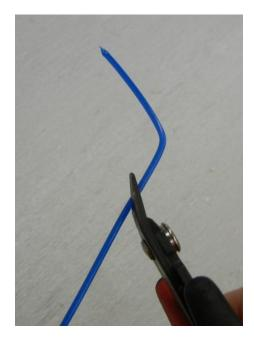
Figure 16: Trim the End of the Filament
