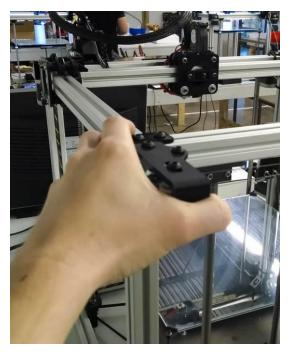
Figure 46: Re-aligning Idler Bracket
