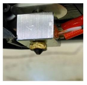
Figure 25: Clean debris-free nozzle
