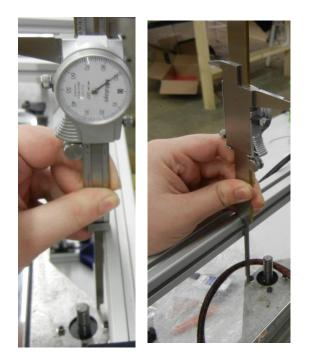
Figure 59: Checking Bed Substrate Level
