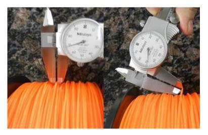
Figure 61: Measuring Filament Diameter
