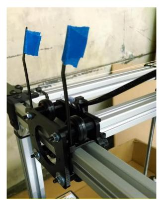
Figure 56: Cut the zip ties flagged with blue tape (qty 4) Open the small box and check the contents against the enclosed packing list.
