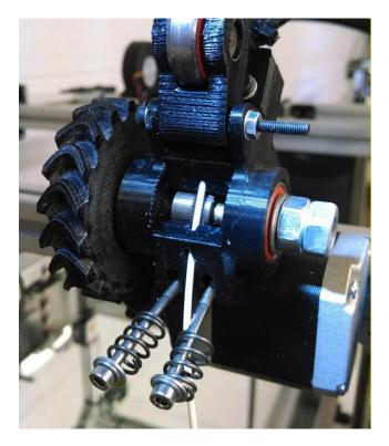
Figure 18: Filament Fed Across Hobbed Gear
