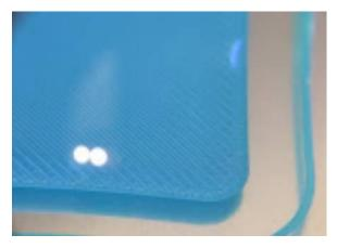
Figure 39: First Layer is Correct
