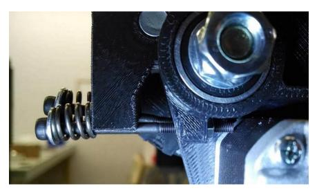
Figure 41: Tips of Bolts Bottomed Out on Motor
