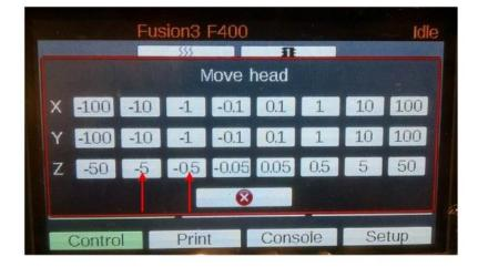
Once the gap gets small use the "-0.05" button to go up in very small increments until you have just a tiny gap between the nozzle and the bed. It can help to shine a light on the wall behind the nozzle like you see in the pictures below.
