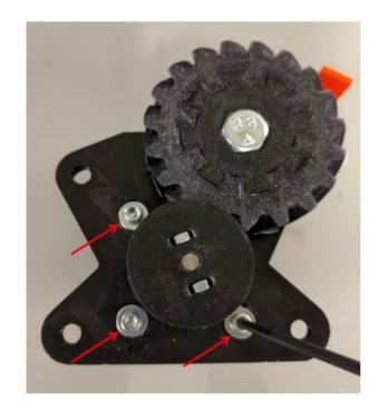
Slide the motor up until the gears mesh firmly. Gently snug the bolts to where the motor will still move when forced.
