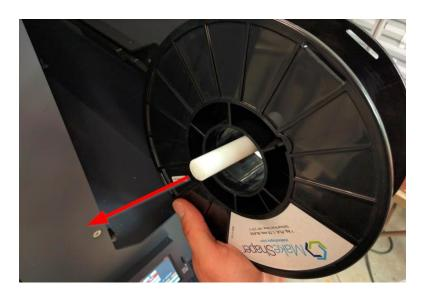
2. Orient the spool so that the filament pays off the front underneath the spool.
