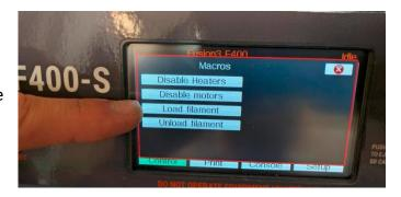
10. After the load is complete the extruder will reverse slightly and the heaters will shut off. **CAUTION**: **The print head will still be hot.**
