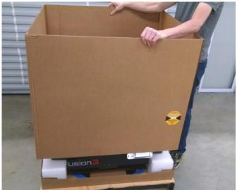
7. Use 2 people to carefully pick up the printer. Lift it out of the bottom tray. The foam endcaps may stay attached – that's ok. Set it on the ground next to the pallet and remove the endcaps one at a time from the printer.
