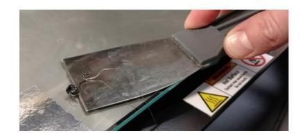
Allow the bed to cool to at least 45°C. Spray water onto the bed using the supplied spray bottle. Let it soak for at least 15 seconds. The glue will turn purple again.
