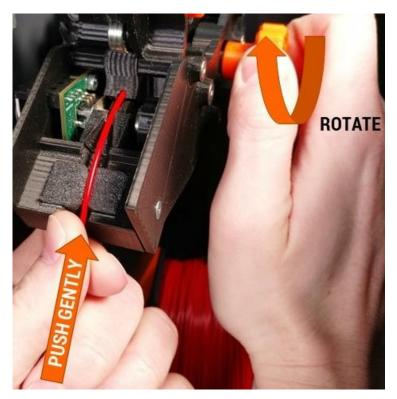
Continue to turn the wheel until the end of the filament protrudes into the feed tube on the exit side of the extruder about 1 inch. Close the Filament Monitoring section.
