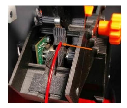
6. While gently pushing on the filament, slowly turn the orange wheel until you feel the extruder "bite" on the filament and begin to pull it. You will see the idler bar "hop" up slightly when this happens.
