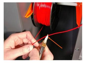
4. Open the Filament Monitoring section of the extruder by pulling towards you on the latch tabs on the Monitoring section door.
