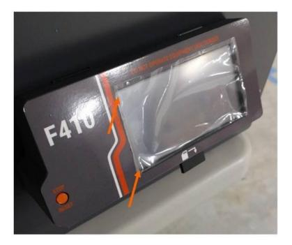
Open the main door and remove the 2 Z axis shipping supports (indicated by orange arrows). One is located near the front of the 3D printer; the other is located towards the center-rear of the F410's print bed.
