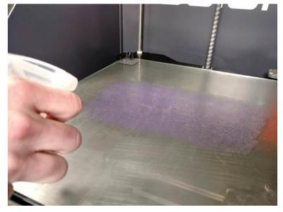
Use your part scraper to "bulldoze" the glue residue into a line. Then wipe up the residue with a paper towel. The bed does not need to be **perfectly** clean, just remove 95% of the gluestick.
