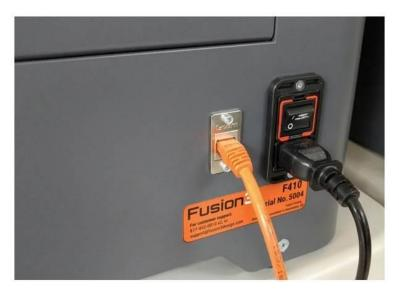
5. Power on your printer using the power switch. Wait 3-5 seconds for it to boot up.
