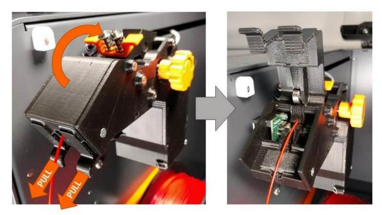
5. Insert the end of the filament into the inlet on the far side of the Filament Monitoring encoder wheel. Push forward gently until you feel the filament bump into the feed gear (inside the feed section).
