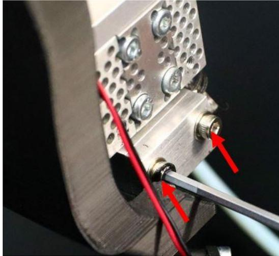
2. Slide the component that needs to be replaced out of the hot block assembly. Disconnect the connector from the print head breakout PCB and trim the zip tie in the bed probe body to free the component.
