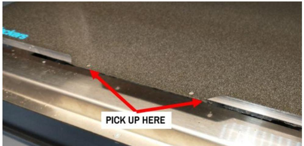
4. Peel it off the bed by lifting the front edge up. Continue to lift it up until all the magnets release.
