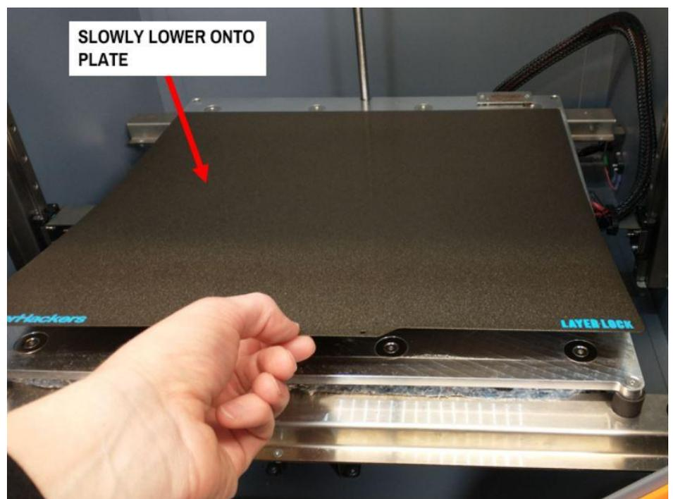
7. For sheets that are smaller than the bed, make sure you leave at least  $\frac{1}{4}$ " overhanging the front of the tool plate, so you can remove the sheet easily.
