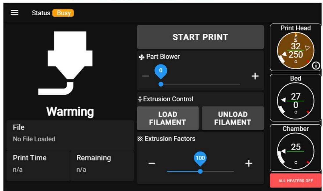
9. Once the head is up to temperature, the extruder will begin to feed filament through the tube and up to the print head. Once the filament reaches the print head, it will extrude out several feet to clear out any old material that might be loaded into it.
