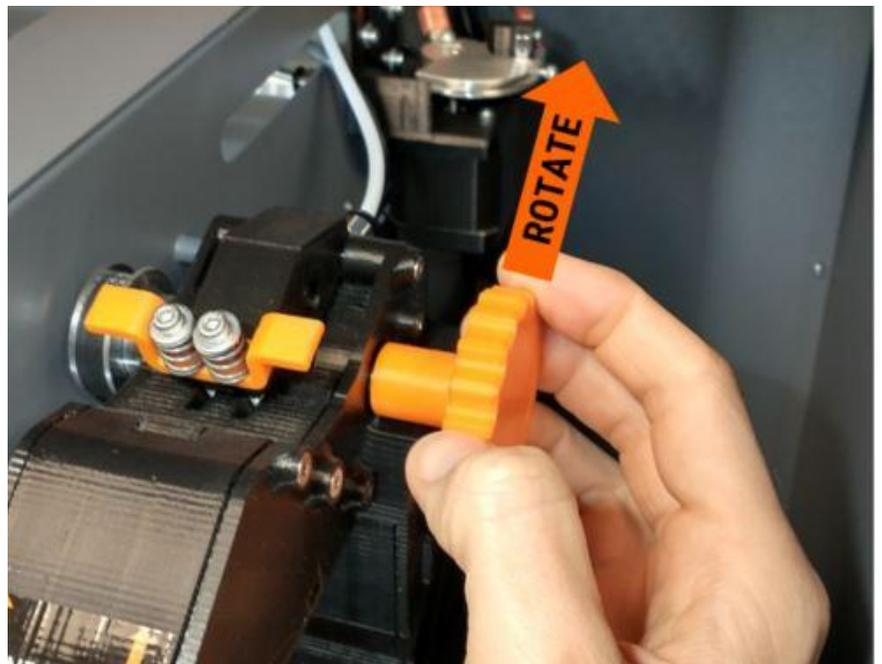
7. Continue to turn the manual advance wheel until you see the filament protrude into the bowden tube at the exit of the extruder. You need to see 1.5-3 inches protruding into the tube.
