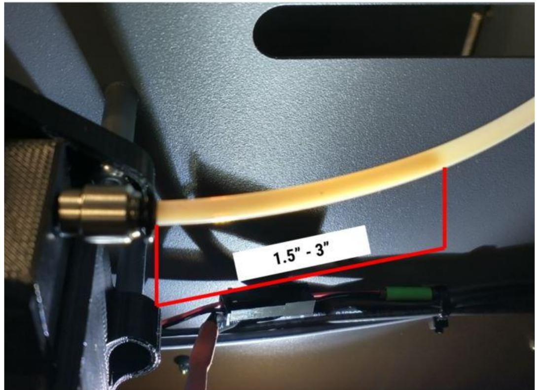
8. On the control panel, select the "Load Filament" button on the main screen. The printer will begin its load filament sequence by heating the head and moving the bed down away from the print head. It can take 1-2 minutes to heat the print head and it will look like nothing is happening; please be patient.
