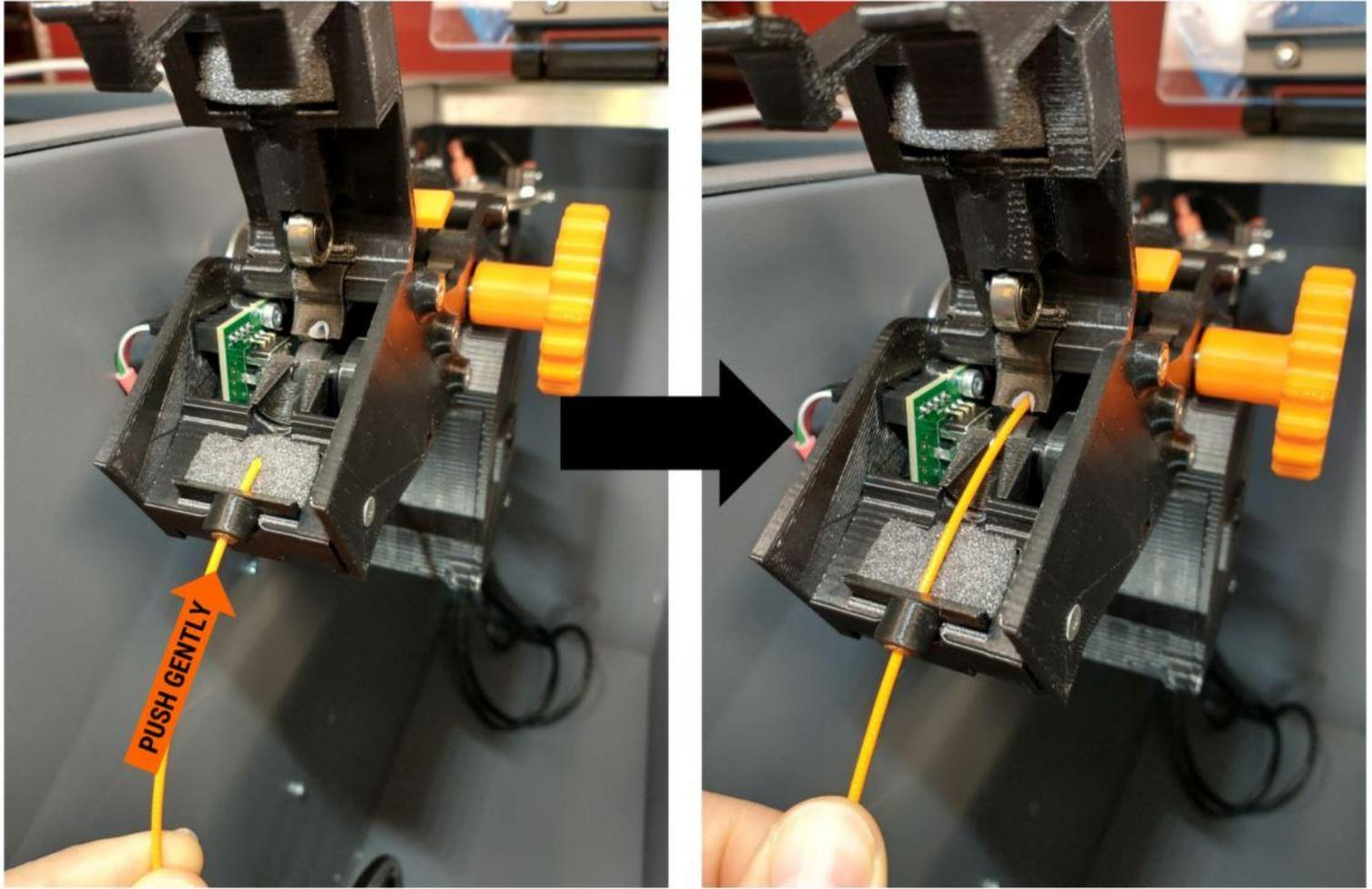
6. Grasp the manual advance knob on the side of the extruder, and rotate it slowly away from you as you continue to push on the filament. You should feel the feed gear engage the filament. When this happens, the idler bar will shift up slightly.
