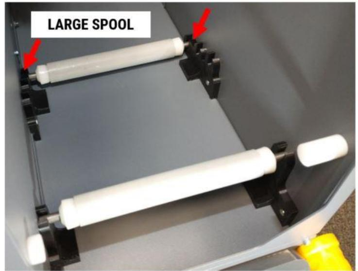
2. Place the filament spool onto the rollers with the free end of filament paying off the front and pointing up.
