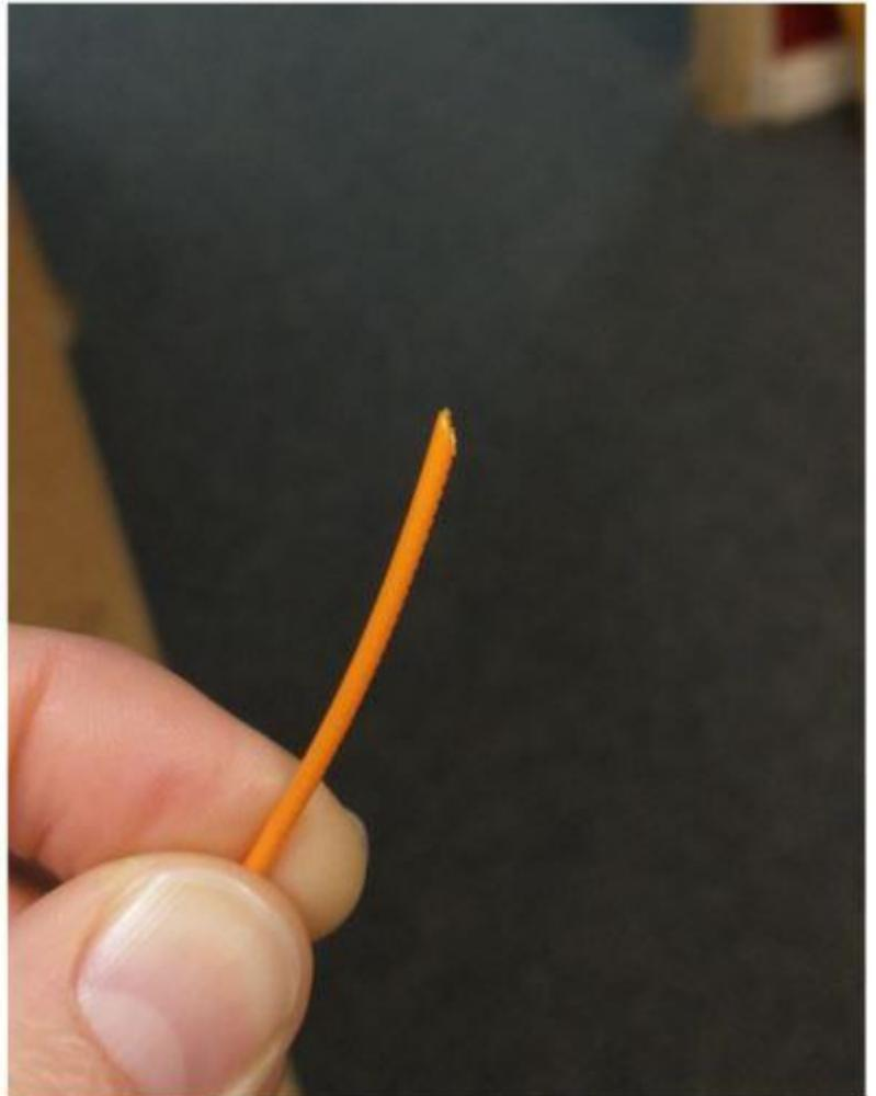
5. Feed the end into the extruder, through the inlet guide, over the wiper, over the monitoring wheel, and into the liner. Gently push until you feel it bottom out.
