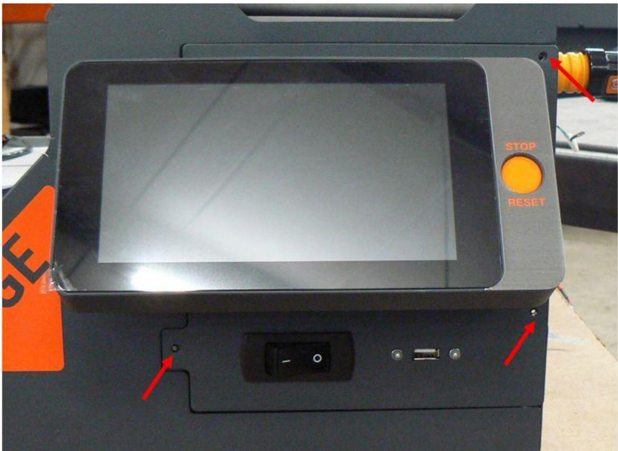
2. SLOWLY and GENTLY slide the sled straight out of the printer. Pause frequently to check for wires that are caught on something, or connectors you forgot to separate. Use the handhold built into the bottom of the LCD bezel for grip. Support the sled from the bottom.
