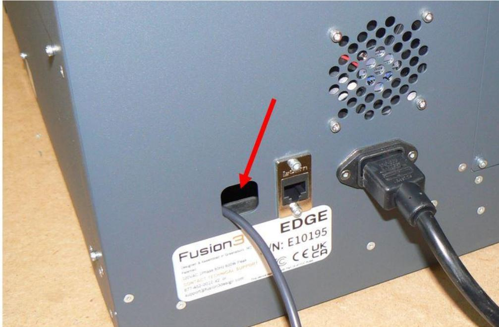
5. **Ground yourself before touching anything in the electronics bay!** Plug the connector into the location shown. The slots in the connector (where metal shows thru) should face you.
