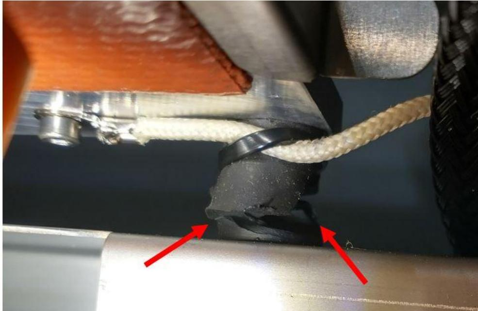
9. If you see the white wire retained to the bed bushing as shown in the picture, please cut the zip tie (be careful not to cut the wire)
