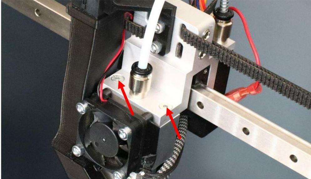
2. Check that the bed probe body screws are tight and the bed probe body is straight up and down
