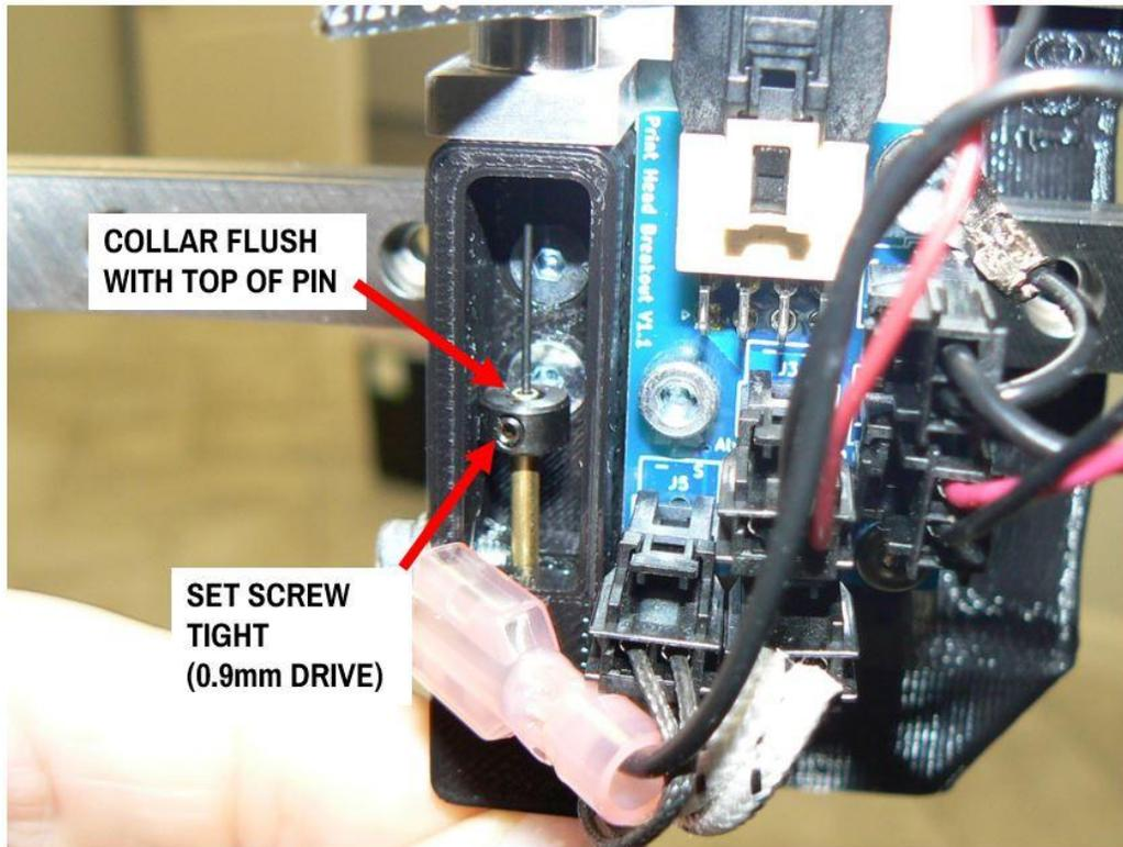
4. Check that the bed probe pin is straight and deploys smoothly (rotate bed probe motor by hand)
