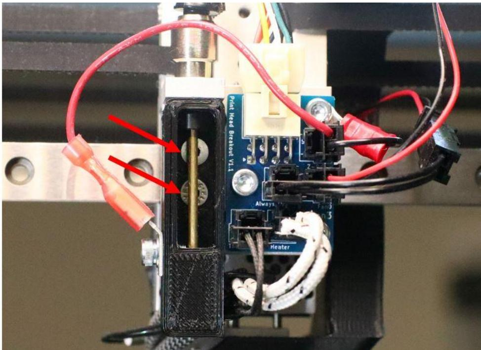
3. Check that the probe pin collar is firmly locked in place and positioned at the top of the pin. Make sure the collar is square relative to the pin (not sitting cockeyed).
