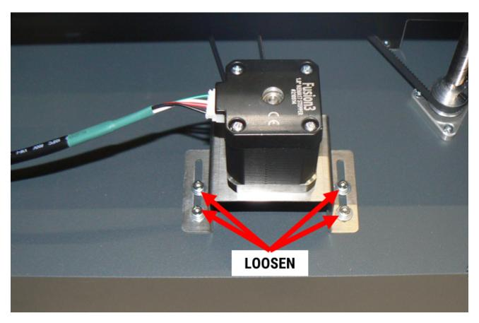
3. Firmly pull the mount to the rear of the machine and retighten the screws.
