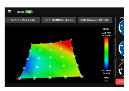
If the printer detects a difference in bed height (max-min) of more than 2.0 mm, it will stop the print and prompt you to manually level the bed.
