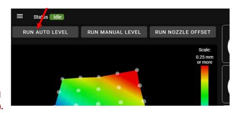
If you need to run the auto bed level outside of a print, use the "Run Auto Level" button on the Bed Leveling screen.
