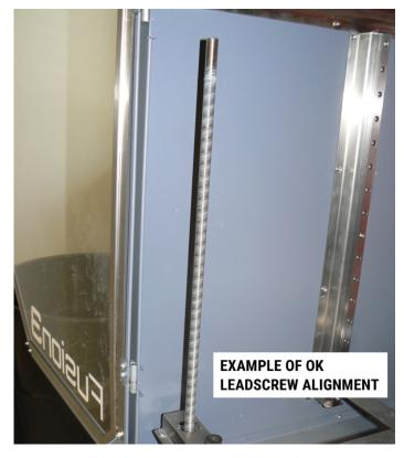
13. Manually raise the Z axis by pulling on the belt, until it's high enough for you to manipulate the manual leveling thumbscrews.
