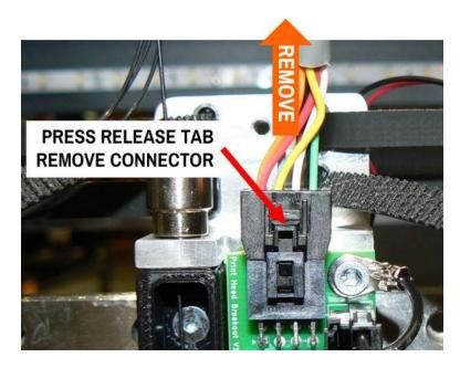
4. Unplug the electronics bay end from its matching connector. This end also has a latch.
