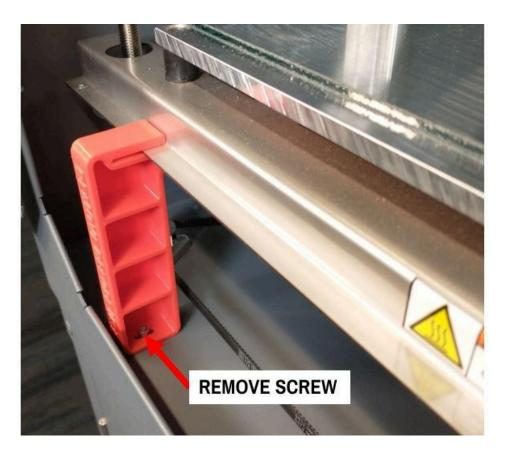
3. Slide the fixtures off of the front edge of the Z axis. You may need to lift the Z axis slightly by moving the belt as shown in the picture.
