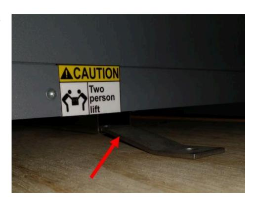
9. Use 2 people to carefully pick the printer up off its pallet and move it to a suitable location.
