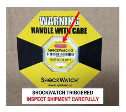
**If the shockwatch is triggered:** Your shipment has experienced a shock > 25G. Your printer may be fine, but the odds of shipping damage are higher.
