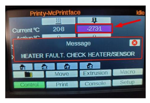
If the open circuit is intermittent, you might see this error, but when you check on the printer later you see a "real" temperature on the screen.
